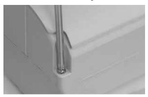
Fig. 4.2.9: Removing screw at the end of casing
