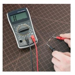
Fig. 1.5.6: Measurement of resistance
