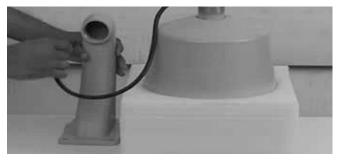
Fig. 4.2.21: Inserting cables through wall mount
