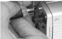
Fig. 4.2.9: Adjusting position of lens
