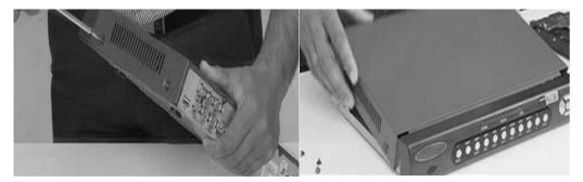
Fig. 5.1.4: Removing the cover of DVR unit
