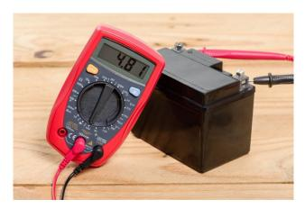
Fig. 1.5.4: Measurement of DC voltage
