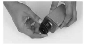
Fig. 4.2.8: Fixing the lens
