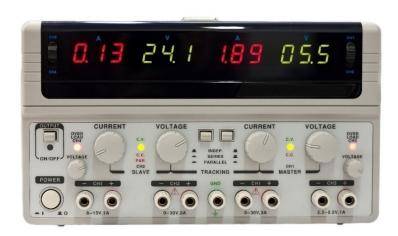
Fig: 1.1.14: Programmable power supply
