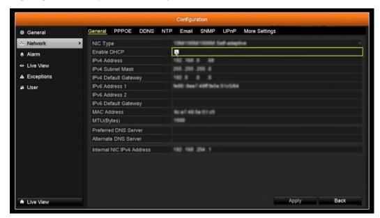
Fig. 5.1.17: Configuring DVR to be operated remotely
